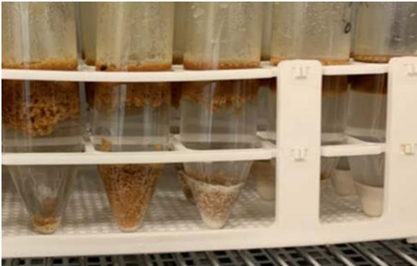
At ESaI, we have chosen modified flotation because of its accuracy and speed of results. A typical salinity series is shown in the photo above where the salinity in each sample is different. The photo shows as the salinity is changed the amount of water-wet rock decreases until almost all the rock is oil-wet floating.
