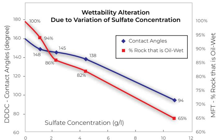
The MFT measurements are compared to contact angle measurements for the same system in the figure above. The results show that the two methods give almost identical results over a wide range of wettability.
